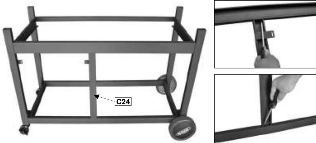
Attach the Front Trim Panel (C24) to the front support and underframe using ST4.0x10 Screws (D1x4pcs) as shown.
