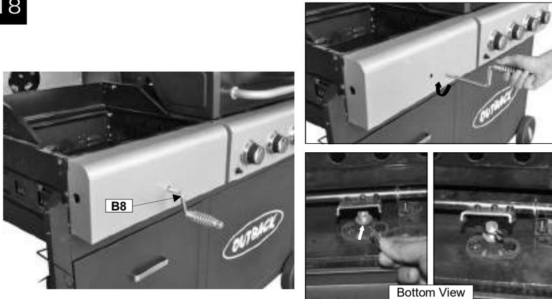
Insert the Crank Handle (B8) through the hole in the Charcoal Control Panel (B7) and screw it into the threaded socket, then secure with a R-Clip (D10) as shown.
