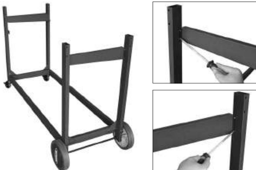
Carefully turn the trolley assembly up. Attach the Drip Tray Left Bracket (C6) to the left legs using ST4.0x10 Screws (D1x4pcs). Repeat above process for fixing the Drip Tray Right Bracket (C8) to right legs.
