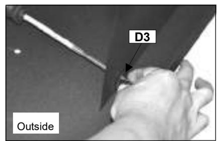
Attach the Charcoal Bin Front Panel (C23) onto the charcoal bin assembly using M4x8 Bolts (D2x6pcs) and M4 Nuts (D3x6pcs) as shown.
