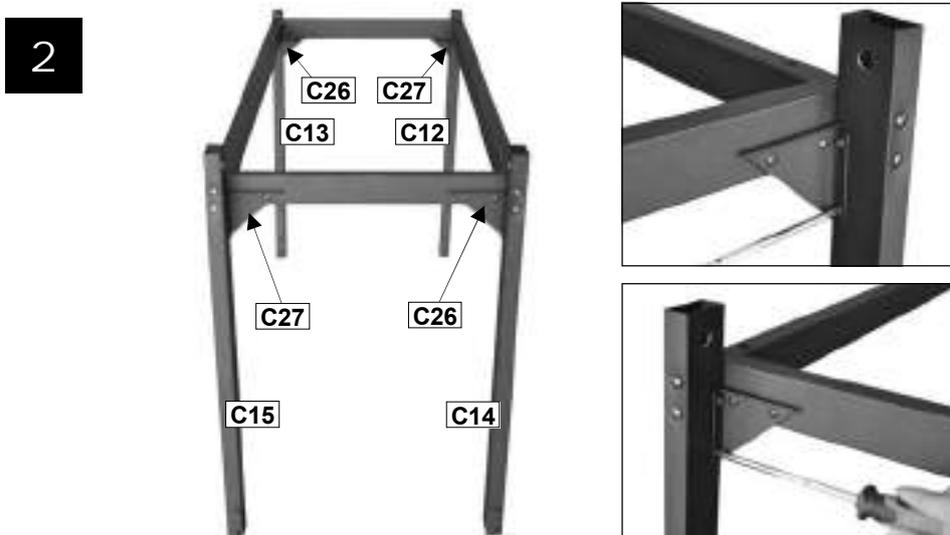
Carefully turn the trolley assembly upside-down.
