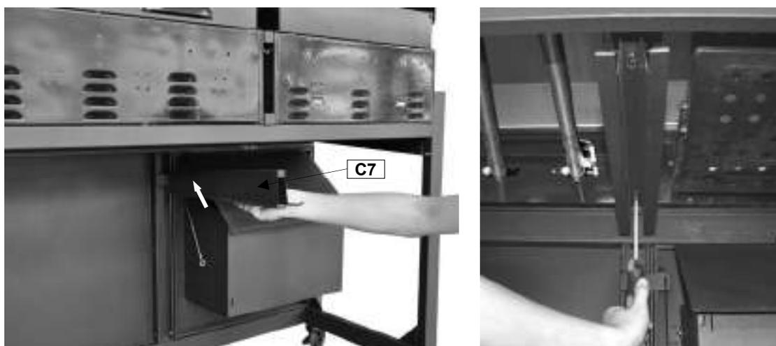
Attach the Drip Tray Middle Bracket (C7) to the barbecue body using M6x15 Bolts (D5x2pcs) as shown.
