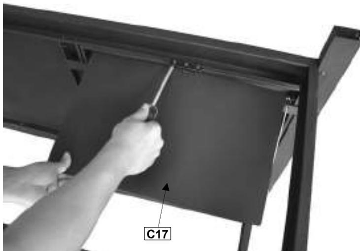
Attach the Charcoal Bin Lid (C17) to the front support using ST4.0x10 Screws (D1x3pcs) as shown.
