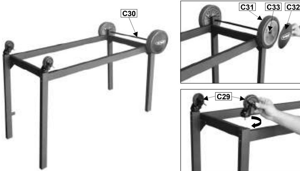
Unscrew the Locknuts (C33) from both ends of the Axle (C30). Slide the axle through the corresponding holes in the right legs. Slide the Wheels (C31) over each end of the axle. Secure the wheels into place with the locknuts. Place the Wheel Hubcaps (C32) onto the outside of the wheels. And attach the Lockable Casters (C29) into the left legs.
