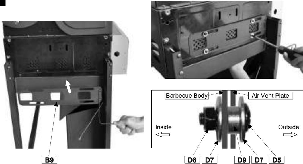
Attach the Air Vent Plate (B9) to the barbecue body using M6x15 Bolts (D5x4pcs), Spacers (D9x4pcs), Ø6 Washer (D7x8pcs) and M6 Nuts (D8x4pcs) as shown.
